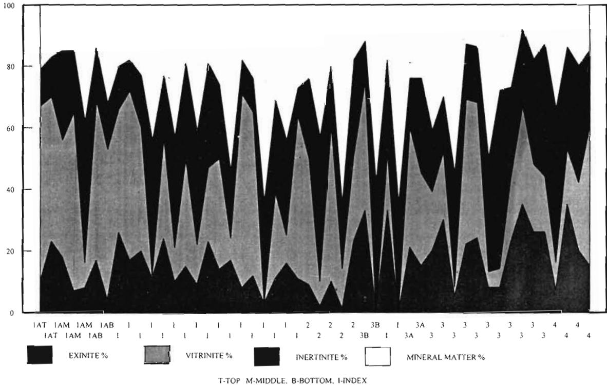
Text-figure 2—Maceral composition of coal seams from Bore-hole no. 732, Ramagundam Coalfield.
