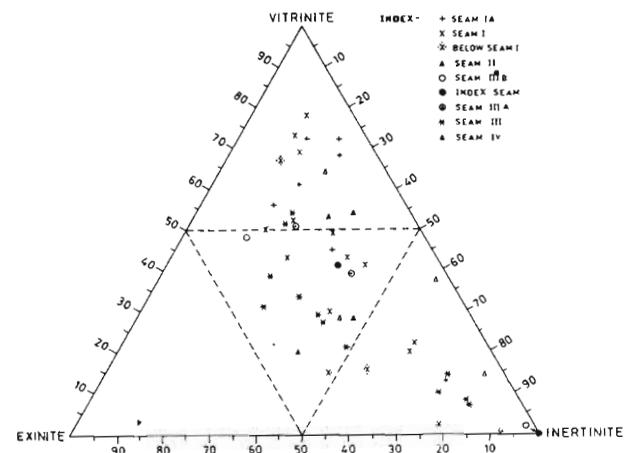
**Text-figure 4**—Triangular data (m.m.f.) of vitrinite, exinite and inertinite macerals in different coal seams of Ramagundam Coalfield.
