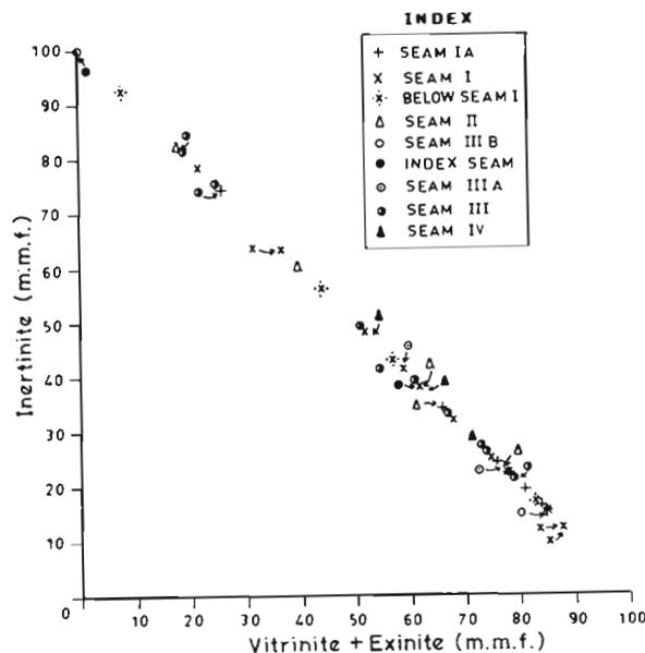
**Text-figure 5**—Biaxial (m.m.f.) maceral data plotting of different coal seams of Bore-hole no. 732, Ramagundam Coalfield.
