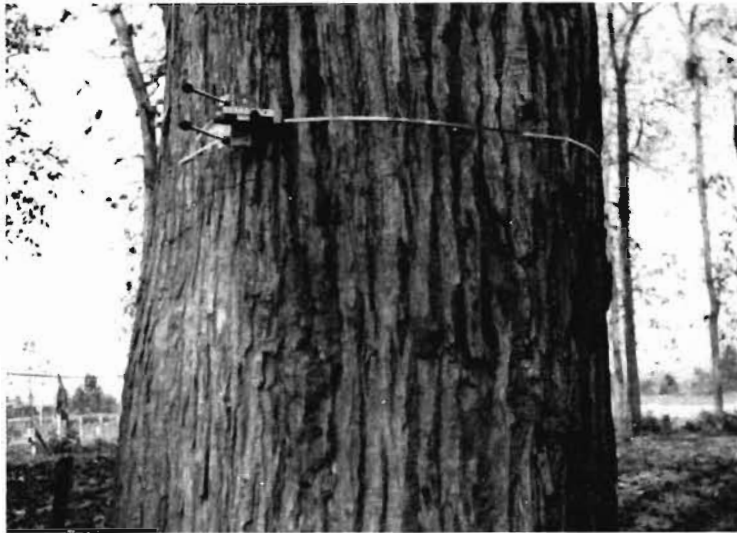
Fig. 2—A Gensler manual band dendrometer on a teak tree at MNFPU
