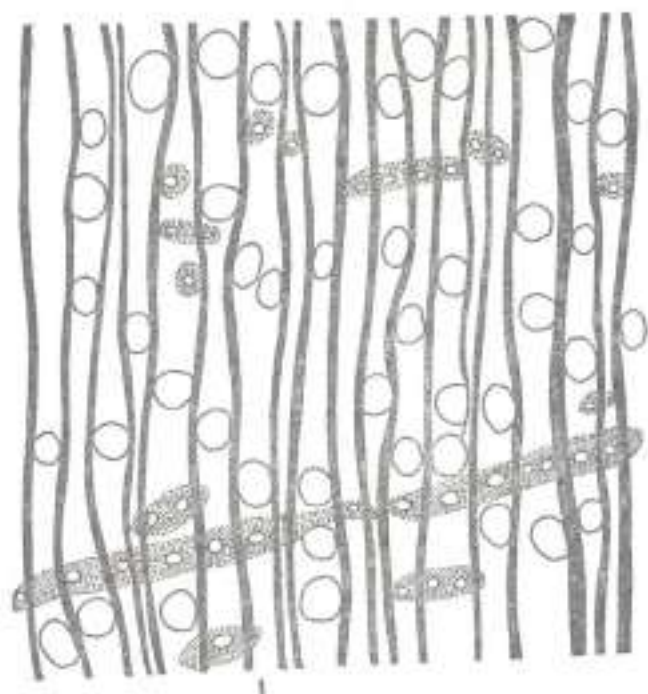
TEXT-FIG. 1—Cross-section showing nature and distribution of gum canals. \times 25 .
